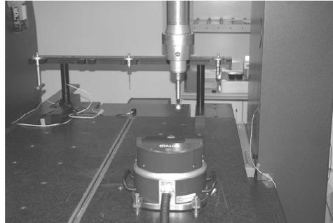
Fig. 1. Cooperation between the CMM and LaserTracer.
