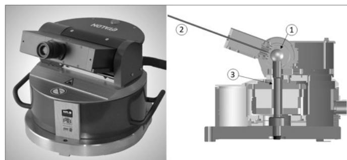
Fig. 2. LaserTracer: 1) reference sphere, 2) laser beam, 3) LT column [28].
