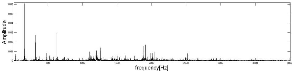
Fig. 3. Fourier spectrum of a typical wind turbine.
