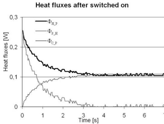
Fig. 6. The heat flux  $\Phi_{H-P}$  that flows into the upper part of a Peltier micromodule. The heat flux  $\Phi_{P-H}$  that flows through the thermal resistance of a Peltier micromodule to the heatsink. The heat flux  $\Phi_{C-P}$  that flows into the body of Peltier micromodule with heat capacity  $C_P$ .
