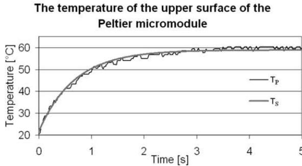
Fig. 4. Temperature of the upper surface of the Peltier micromodule after turning on.  $T_P$  - temperature measured using the Seebeck voltage,  $T_S$  - temperature simulated in Multisim program based on the model without a finger.
