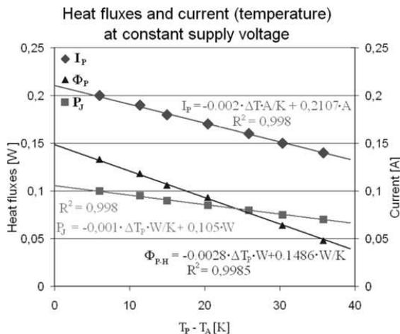
Fig. 5. Values of current  $I_P$ , power  $P_J$ , and heat flux  $\Phi_{H-P}$  pumped by the Peltier micromodule as a function of temperature difference between hot and cold side of Peltier micromodule. The supply voltage equals 0.5 V.
