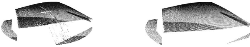
Fig. 6. Free form surface scanning result without (a) and with (b) the use of predictive algorithm.
