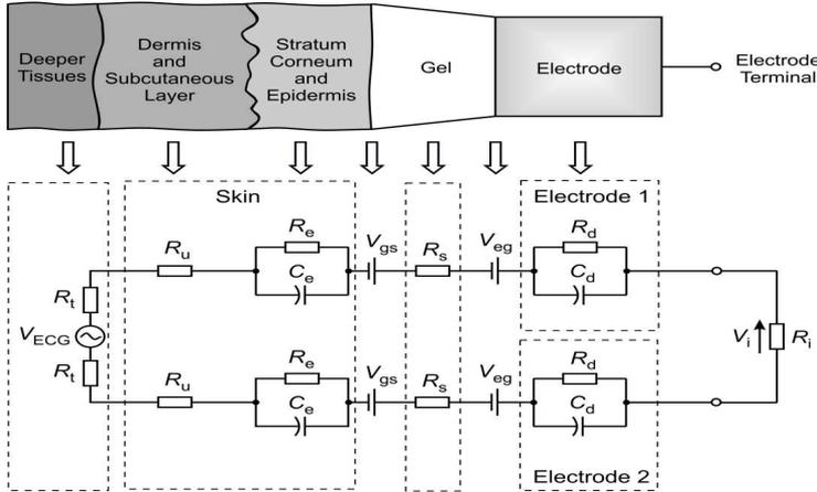
Fig. 3. Skin-electrode interface and its electrical equivalent circuit.
