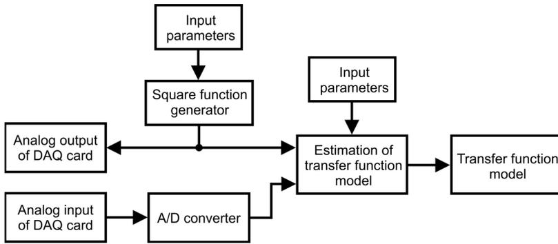
Fig. 5. Block diagram of program for skin-electrode interface identification.
