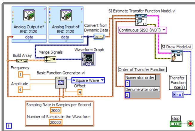
Fig. 6. Program for identification of skin-electrode interface implemented in LabVIEW.
