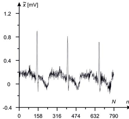
Fig. 10. Signal  $\tilde{x}(n)$  reconstructed on skin-electrode interface input.
