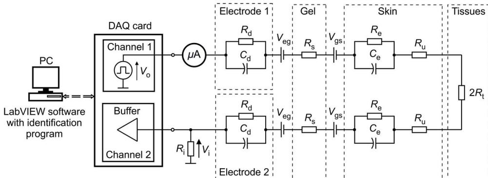
Fig. 4. System for identification of the skin-electrode interface.
