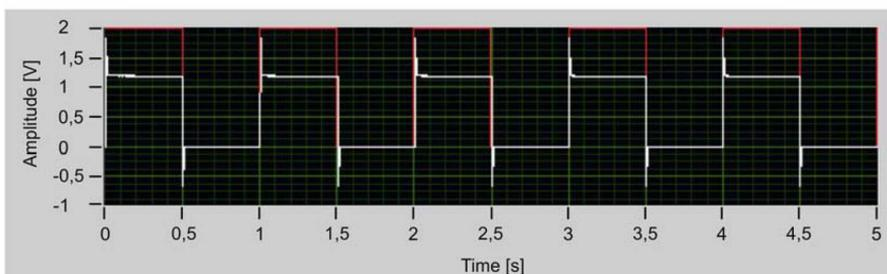
Fig. 7. Wave form of signal across the skin-electrode interface circuit in response to a square stimulus signal.
