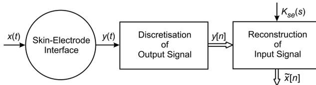
Fig. 2. Block diagram for correction of the error of the signal registered at the interface output
