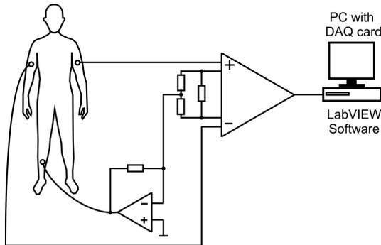
Fig. 8. System for signals registration at the skin-electrode interface output.
