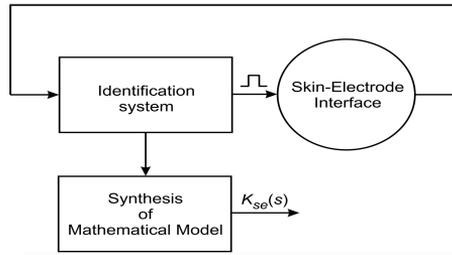
Fig. 1. Block diagram of procedure for identification of skin-electrode interface
