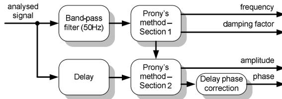
Fig. 2. The idea of precise fundamental harmonics estimation.
