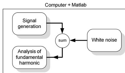
Fig. 6. Waveform generation and analysis system.
