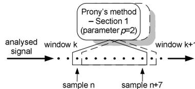
Fig. 3. Prony’s method for fundamental harmonics estimation.
