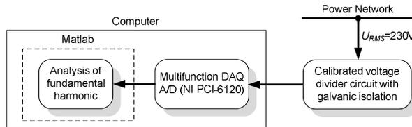
Fig. 8. Power waveforms acquisition system.
