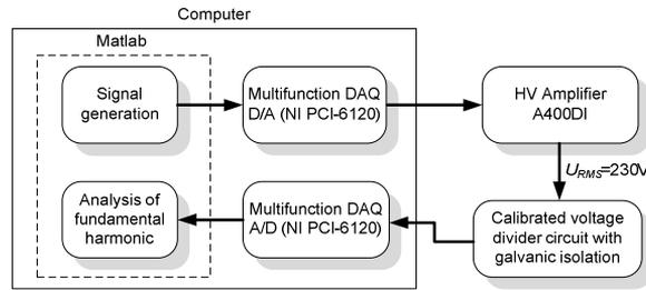
Fig. 7. Power waveforms generation and acquisition system.
