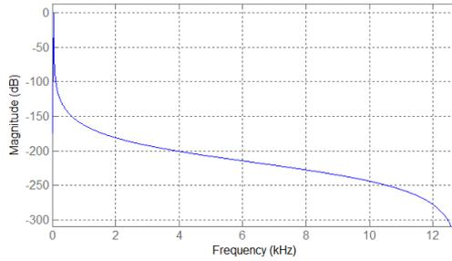
Fig. 4. Magnitude response of band pass filter.
