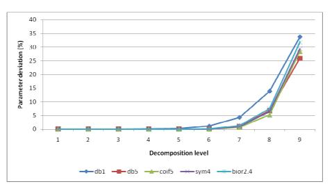
Fig. 2 Relative changes in  $Z_q$  during wavelet approximation for roundness profiles (sample: n = 100 profiles).
