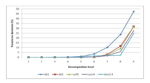
Fig. 5 Relative changes in  $Z_t$  during wavelet approximation for roundness profiles (n=100 profiles).
