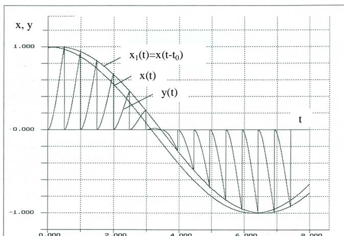
Fig. 3. The input signal  $x(t) = \cos 0.5t$ , the perfectly delayed input signal  $x_1(t_0)$  and the output signal  $y(t)$  of an expanding system based on transducer (15) with  $B = 3$ .
