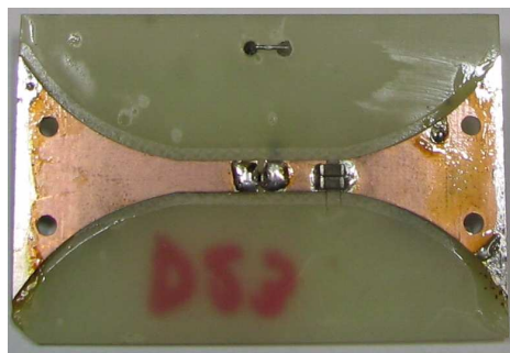
Fig. 5. View of the bottom side of the planar structure of the microwave multiplication system with transformers.
