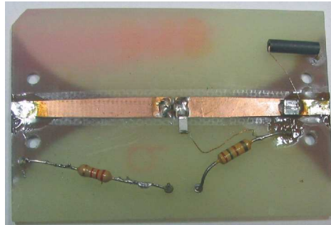
Fig. 4. View of the upper side of the planar structure of the microwave multiplication system with transformers.
