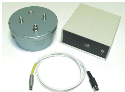
Fig. 5. The 1 GΩ standard developed at INRIM with its external temperature control.
