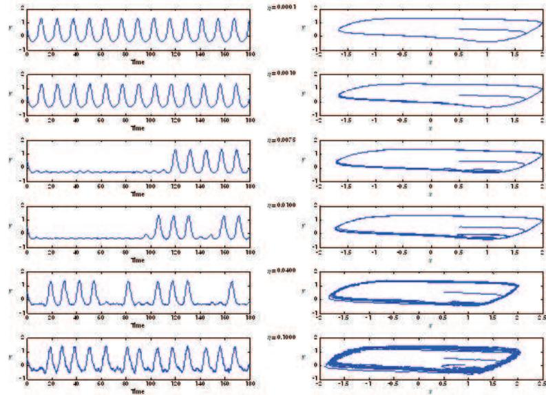
Fig. 3. Outputs  $y(t)$  and phase portraits  $(x, y)$  for the BvP model for  $z = -0.340$  and various levels of perturbations  $\eta$ .
