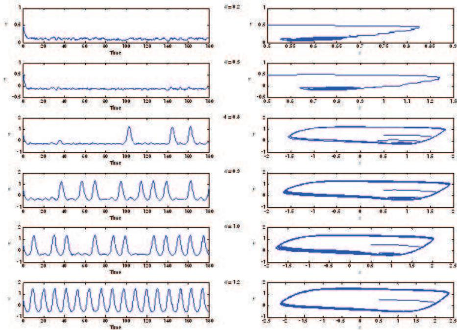
Fig. 1. Outputs  $y(t)$  and phase portraits  $(x, y)$  for the BvP model as a function of  $d$ ; during all simulations  $z$  was set equal to  $-0.340$ .
