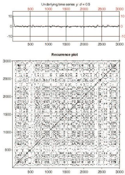
Fig. 6. Time-series  $y(t)$  and recurrence plot for the BvP model; conditions as in Fig. 1 ( $d = 0.5$ ).
