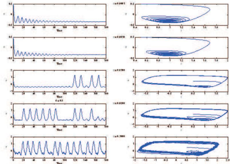
Fig. 4. Outputs  $y(t)$  and phase portraits  $(x, y)$  for the BvP model for  $z = -0.345$  and various levels of perturbations  $\eta$ .
