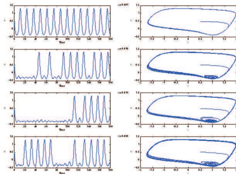
Fig. 2. Outputs  $y(t)$  and phase portraits  $(x, y)$  for the BvP model for  $z = -0.335$  and various levels of perturbations  $\eta$ .
