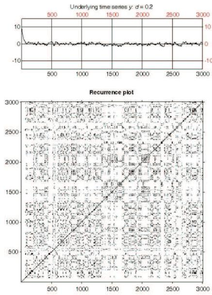
Fig. 5. Time-series  $y(t)$  and recurrence plot for the BvP model; conditions as in Fig. 1 ( $d = 0.2$ ).
