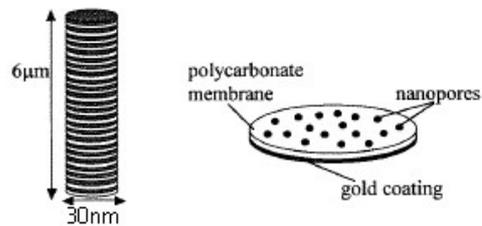
Fig. 2. Schematic diagram of a gold-coated (on the back side) polycarbonate membrane.
