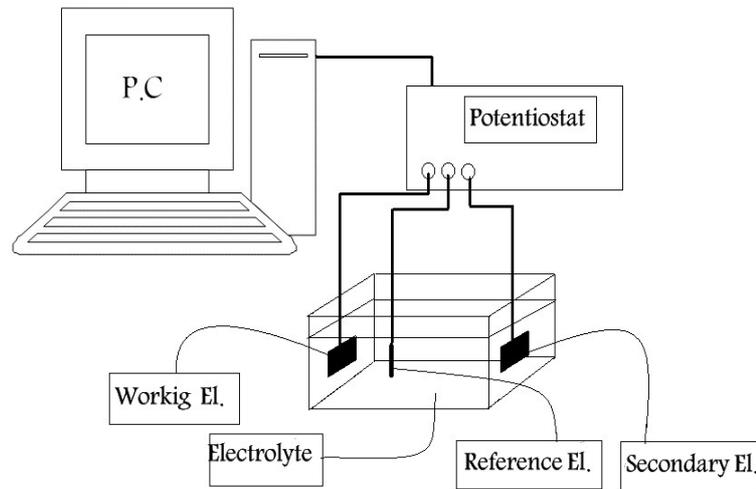
Fig. 1. Experimental set-up for electrodeposition of multilayer nanowires.
