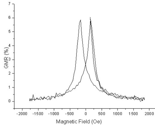
Fig. 7. Percentage change in the giant magnetoresistance as a function of magnetic field for a Co/Pt nanowire.
