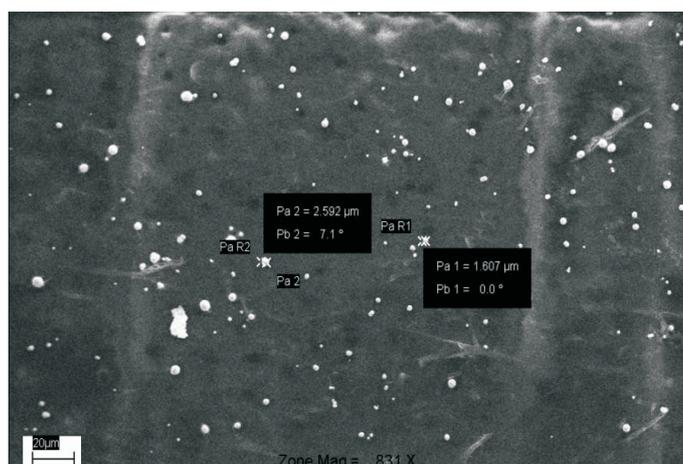
Fig. 3. SEM image of a polycarbonate membrane filled with nanowire.
