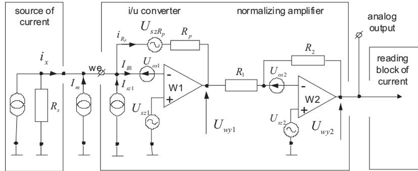
Fig. 5. Scheme of the picoammeter with an active  $i/u$  converter and with the most important sources of disturbances pointed out.
