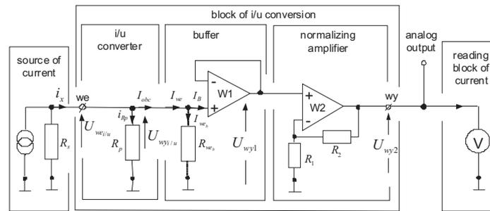
Fig. 3. Schematic diagram of a picoammeter with a passive i/u converter.
