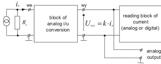
Fig. 1. Block diagram of a picoammeter with analog i/u conversion.
