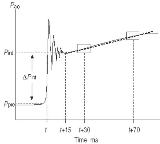
Fig. 2. Schematic diagram illustrating calculation of the interrupter pressure.
