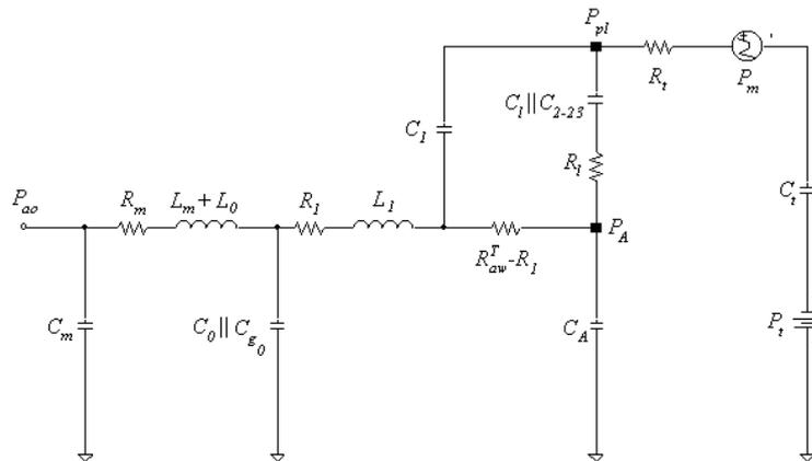
Fig. 4. Metrological model of the respiratory system during airflow interruption [39].
