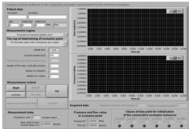
Fig. 6. The main panel of the program for the occlusional data acquisition.
