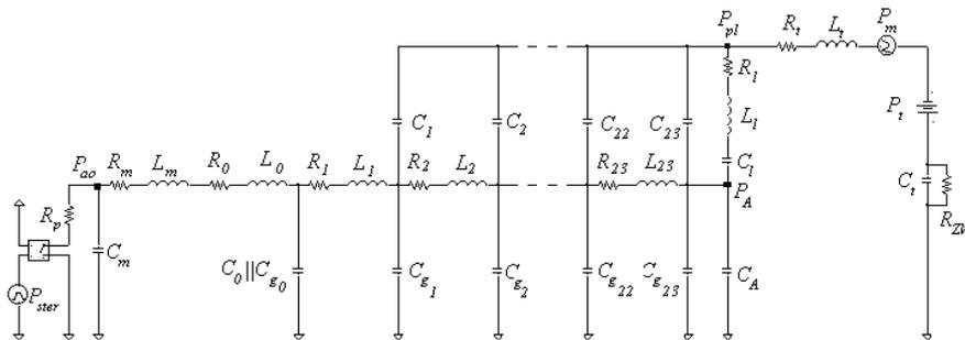
Fig. 3. Linear electrical replacement model of the respiratory system during airflow interruption [38].
