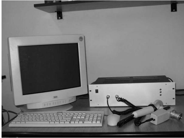
Fig. 5. The station for interrupter data acquisition for the evaluation of respiratory mechanics.
