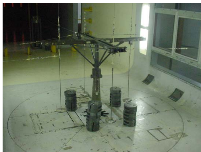
Fig. 2. Loading system for the balance calibration.
