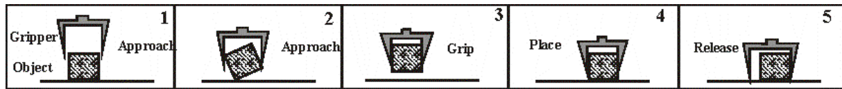
Fig. 7. Typical pick-and-place assembly in microscale. 1). A gripper approaches to a component. 2). The component sticks to the gripper. 3). The gripper grasps the component. 4). The component is transported to a desired location. 5). The component is placed at inaccurate position, component sticks to the gripper.
